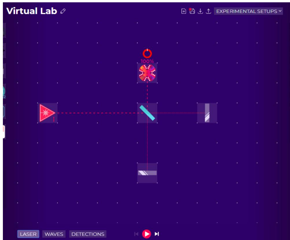
Move the DETECTOR one step/block away from the LASER beam. The DETECTOR number should stay unchanged.
