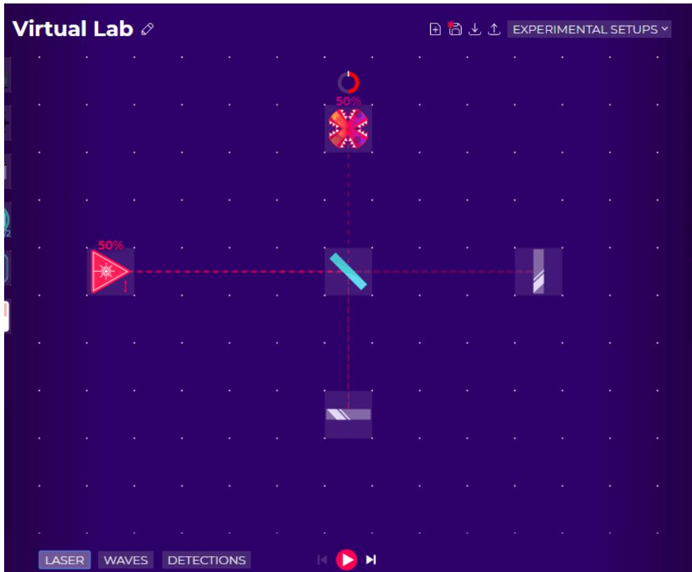
Move the bottom MIRROR one step/block away from the LASER beam.
