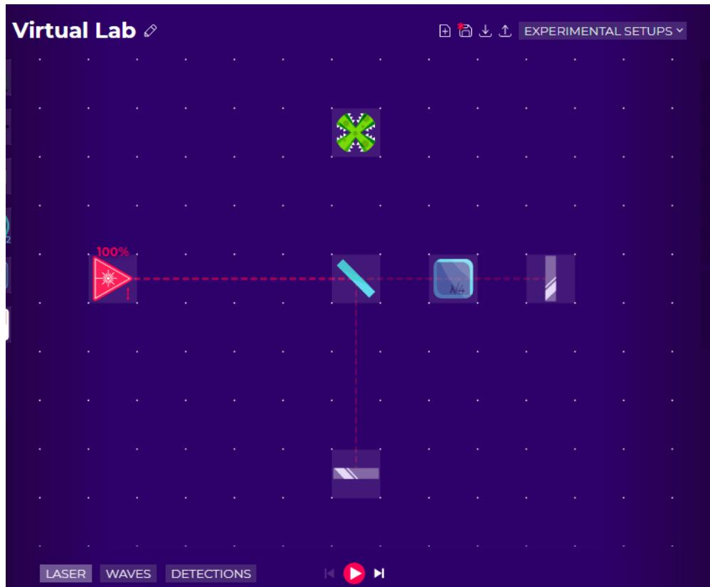
The default phase shift of the GLASS is  $0.25 \times \text{wavelength} (\lambda)$ . It must be visible on the GLASS icon.
